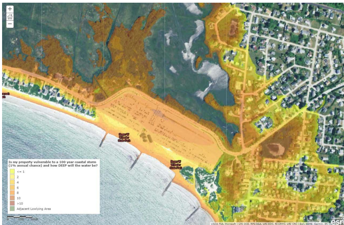
Figure 1. Present-Day Scenario (100-year return period storm surge, no sea level rise) at Roger Wheeler State Park, Narragansett, RI. Colors represent flooding in feet with darker orange representing deeper water. Flooding across the dark section of the beach parking lot in this picture is approximately 7 feet deep. Shades of orange and yellow are used in this figure to represent risk under present day conditions. Map created using STORMTOOLS.
