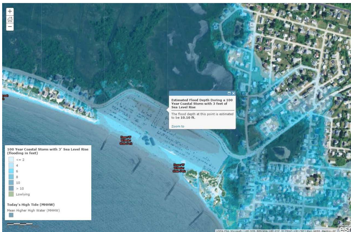
Figure 2. Mid-century Planning Scenario (3-foot sea level rise plus a 100-year return period storm surge) at Roger Wheeler State Park, Narragansett, RI. Colors represent flooding in feet with darker blue representing deeper water. Flooding across the darkest section of the beach parking lot in this picture is greater than 10 feet deep. Shades of blue are used in this map to represent risk under future conditions, as opposed to shades of orange which are used in other figures to represent present day conditions. Map created using STORMTOOLS.
